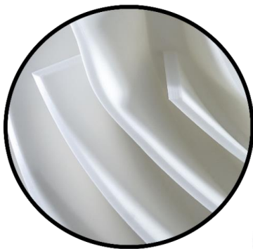
Close up a printed object with Strong PLA (Printed on an Ultimaker 2+, 0.19 layer height, 242°C)
