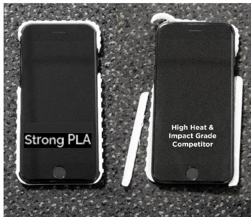
3D printed iPhone 7 cases (after annealing at 110°C / 20min)
