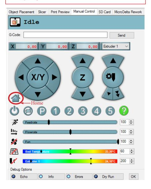
2°) Make sure that EVERY sliders move up till hitting it's corresponding endstop.
