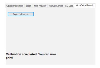
The calibration process is meant to be done once and not before every print. In some cases, the calibration could become unaccurate, after disassembling and reassembling structural parts of you printer per example, you should then calibrate again your printer.
