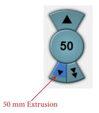
2°) Verify that melted filament comes out of the nozzle regularly.
