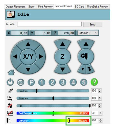
If the target temperature is not reached or the actual temperature varies a lot around the target temperature, perform a PID calculation (see appendix).
