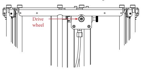
5°) Tighten the spring strongly by turning the knurled screw. Note: if the thumbwheel is not tight enough, the filament will be badly driven.
