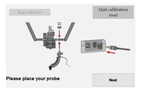
3°) By clicking «Next», the calibration begins and calibration module will start it's multi-point bed probing. This process can take several minutes.
