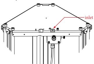
4°) If you encounter a hard point while inserting the filament, engage the extruder and turn the drive wheel until the filament gets to the nozzle, melted filament should start coming out
