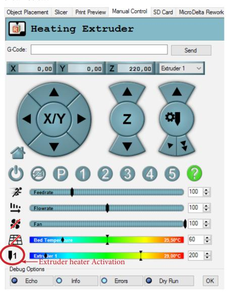
2°) Check that the target temperature is reached:
