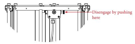
3°) Insert the filament in the extruder's inlet and push it as far as possible
