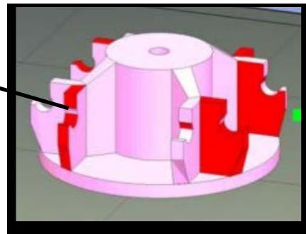
After selecting the model, choose Edit - Fix to repair the model.
