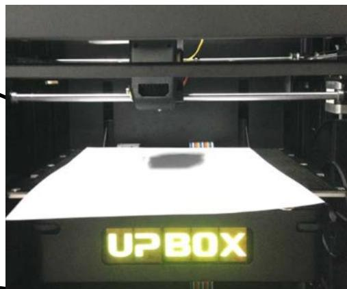
Hit the "5" button. Nozzle will go to the center of the platform.
