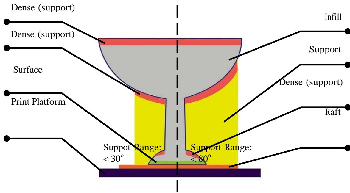
**Dense:** Solid support structure ensure the surface being supported retain its shape and surface finish.
