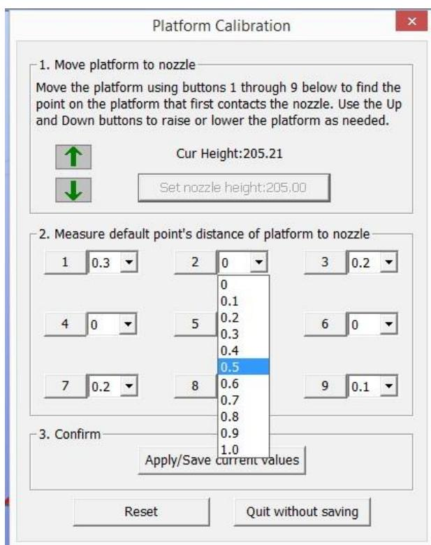
For example, setting the compensation value for calibration point No.3. Assume the "platform height" is 208.7 and the "nozzle height" is 208, the compensation value should be set to 0.7.
