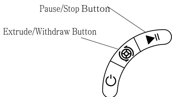
Alternatively, during Printing, double click the Pause/Stop button, the print job will be paused. It is possible to use the Extrude/Withdraw button to change filament during pausing. Double click the pause/stop button again to resume the print job.
