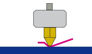
Platform too high, nozzle is pinning paper onto the platform. Lower the platform slightly.
