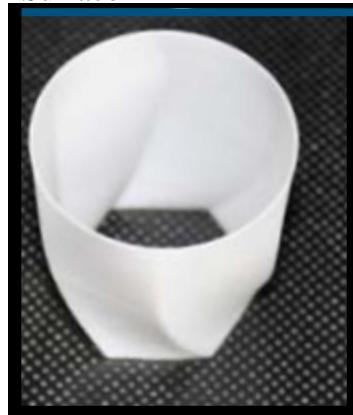
The object will be printed without bottom layers and top layers. Only a surface with single layer thickness will be made.
