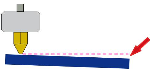
As shown in the left, when platform is at the "nozzle height", only part of the platform is close enough to the nozzle. Therefore we need to set compensation values for all other calibration points to inform the printer about the distance between nozzle and print surface throughout the XY plane.
