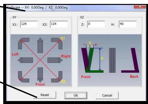
Hit "Reset" button to revert the value back to default, make sure the upper panel display: XY:0.00 Deg/XZ:0.00 Deg
