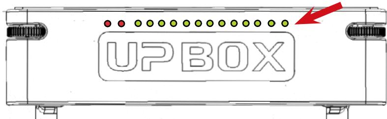
Printing progress is shown in the LED progress bar on top of the UP BOX letters. The first two red LED represent printing of raft, the others represent the rest of the model.
