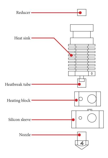
The central tube is attached to the heatsink using a thin weld. It is therefore important to never screw the heat break tube on the heater block by directly hold the heat sink under penalty of breaking this weld.
